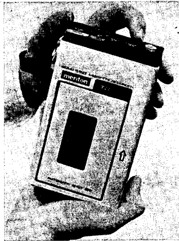
Meriton recorder keeps all controls in line at top. Size and color of buttons make them easily distinguishable.
