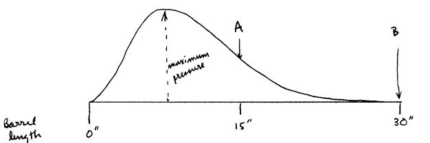
If you fired a rifle with a 30" barrel, the powder would but off by the time your bullet reached point "B", and there would be no smoke emitted from the muzzle. If your barrel were 15" then all the burning that normally would take place inside the long barrel between points "A" and "B", instead takes place in the air in front of the muzzle. Your 15" barrel would produce smoke.
