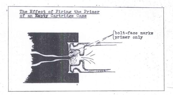
The force of the primer's blow-back causes the primer to be imprinted by the steel bolt#face and firing pin of the rifle in which it is fired. When the pressure falls, the resilient surface of the primer recedes from its tight contact with the steel surface. It now bears a unique set of marks that can have been made by one bolt#face and one firing pin to the exclusion of all others in the world.
